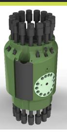
HYDRAULICALLY OPERATED LUBRICATOR VALVE WITH BIDIRECTION PRESSURE SEALING CAPABILITIES. INSTALLED IN THE UPPER LANDING STRING ASSEMBLY TO ISOLATE WELL BORE FROM BELOW AND ISOLATING THE DRILL FLOOR FROM THE WORKOVER RISER.
