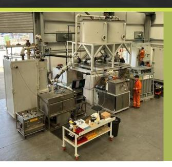
ISE has a comprehensive hydrostatic pressure test facility including temperature, flow loop and hyperbaric testing.
